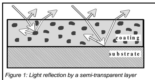
Figure 1: Light reflection by a semi-transparent layer
