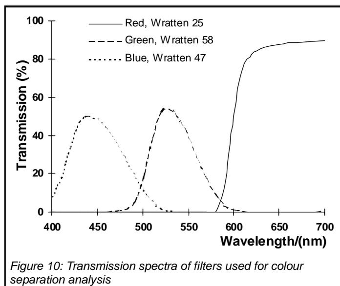
The printing plate for the cyan ink is prepared from the image transmitted through the red filter, as illustrated in Figure 11.
