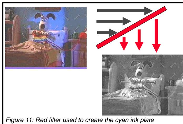
The plate for the magenta ink is prepared using the image transmitted through the green filter and the plate for the yellow ink is prepared using the blue filter. The printing plate for the black ink is prepared using a more or less neutral coloured filter.
