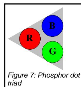
If the space between the phosphors is filled with black, then the impression of a brighter image of higher purity is obtained.
