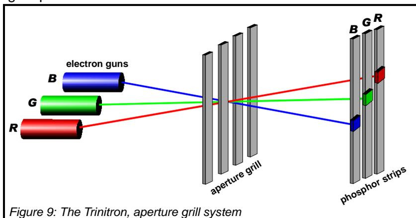
Figure 9: The Trinitron, aperture grill system
