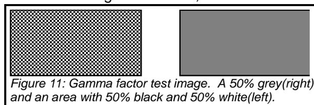
Figure 11: Gamma factor test image. A 50% grey(right) and an area with 50% black and 50% white(left).
