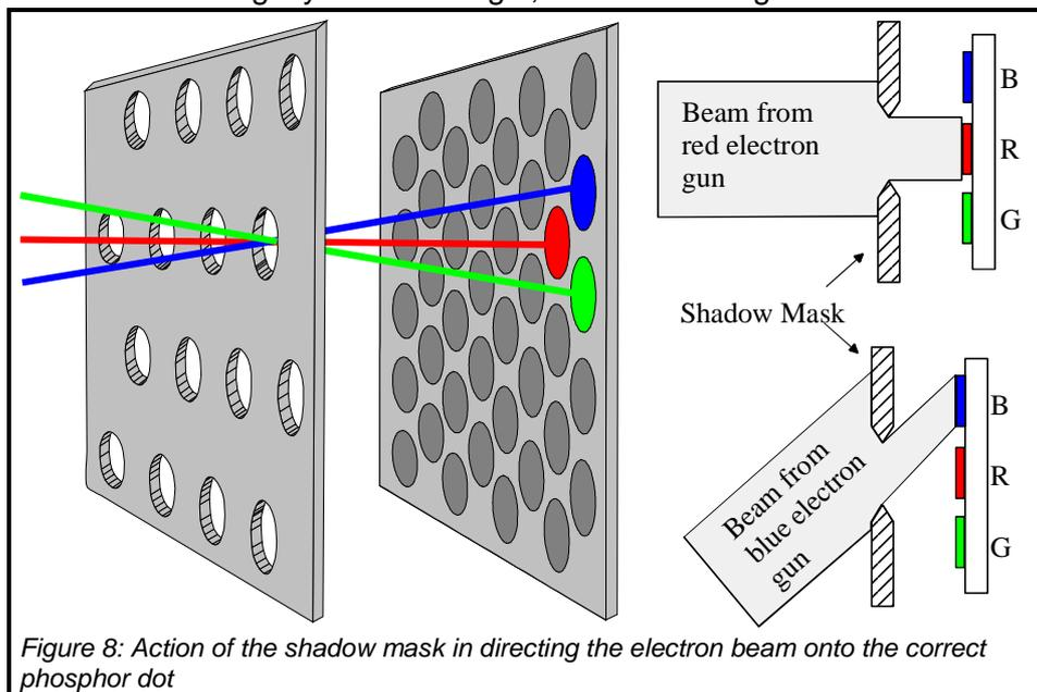
Figure 8: Action of the shadow mask in directing the electron beam onto the correct phosphor dot
