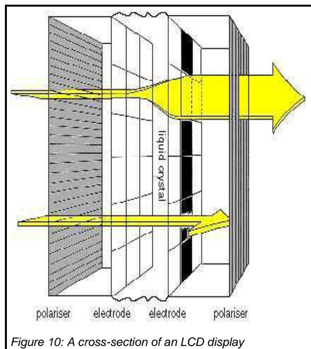
Figure 10: A cross-section of an LCD display
