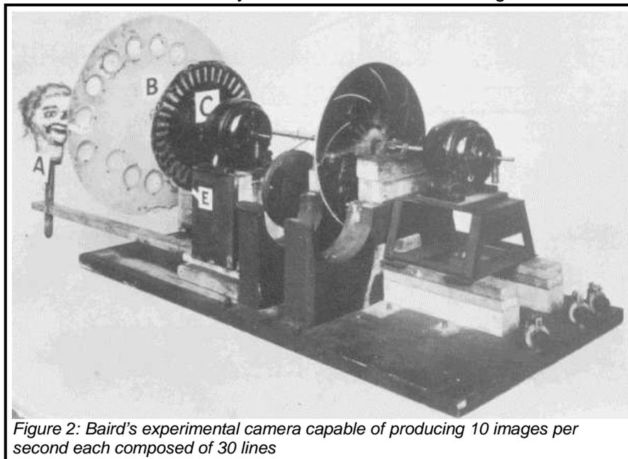
*Figure 2: Baird's experimental camera capable of producing 10 images per second each composed of 30 lines*
