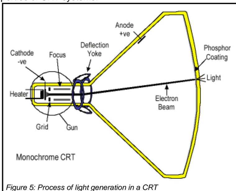
Figure 5: Process of light generation in a CRT
